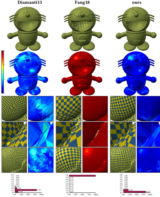
Fig. 5. Robocat. *Top to bottom*: texture, a heat map of the isometric distortion  $\tau$  in (3), three other viewpoints, and a distortion histogram.
