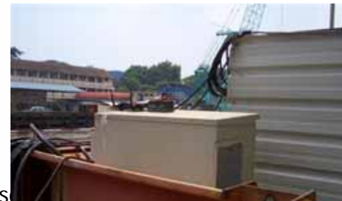
Router 4 being placed on top of metal box and blocked by aluminium wall.
