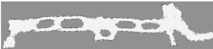
Figure 13. The global gridmap constructed with the new algorithm, by combining the recorded sonar data with the global coordinates generated by the algorithm.
