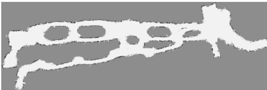
Figure 14. The global gridmap constructed without the new algorithm, by combining the recorded sonar data with the global coordinates calculated using the compass and odometry. Without the algorithm, the robot fails to build a consistent map.
