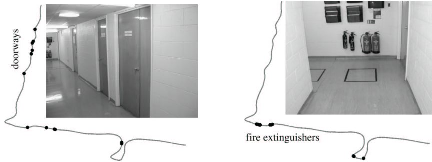
Fig. 2. An example of the differences in landmark selection between the ( left ) standard anticipatory model and the ( right ) GWR non-anticipatory model, a_T = 0.85 . All methods trained using the same parameters on the same data and tested on the same data (different from training set). Landmarks found are shown by black dots on the line of the route path. They correspond to physical features on the route: an alcove, fire extinguishers on the wall ( inset right ), and a series of closed doorways ( inset left )
