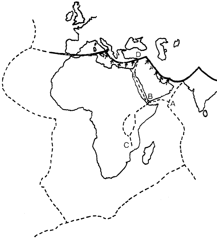
FIG. 2. The African and Arabian plates. Spreading ridges and transform faults are indicated schematically by dotted lines, compressional boundaries by continuous lines, and active subduction zones by arrows.
