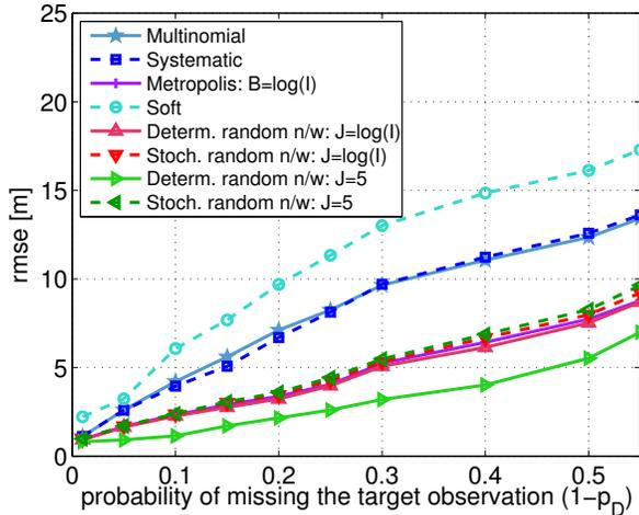
Fig. 9: rmse versus the probability that a sensor misses an observation. The number of particles  $I = 1024$ . The particles are initialised uniformly in the surveillance region, and a burn-in time of 10 seconds is then applied.
