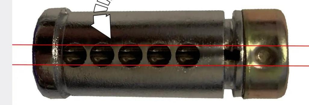
Misaligned holes means that as rotate plug that some pins will get stuck ("bind").
