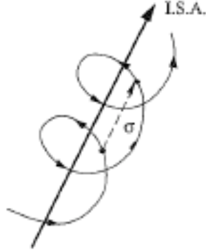
Figure 4.1: The pitch \sigma is the distance travelled parallel to the I.S.A. in one revolution about it
