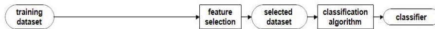
Fig. 3. The training process of classification with incomplete data by using feature selection.
