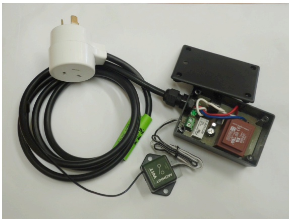
Figure 9. The Mains sensor connected to Monnit Open/Close module
