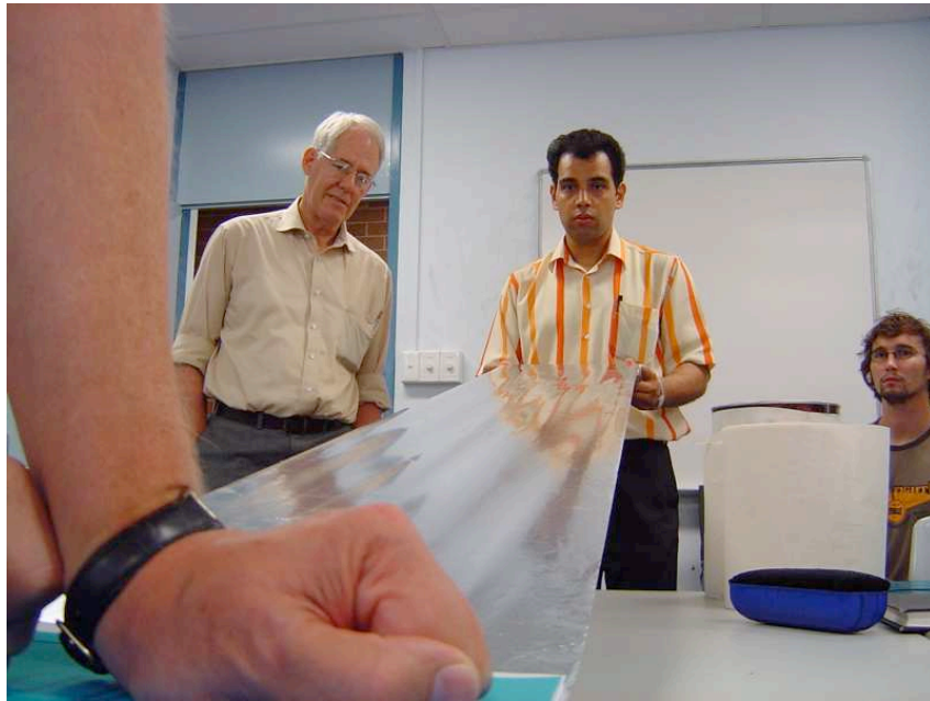
Figure 2: Experiments producing wrinkles in tin foil by stretching lengthwise.
