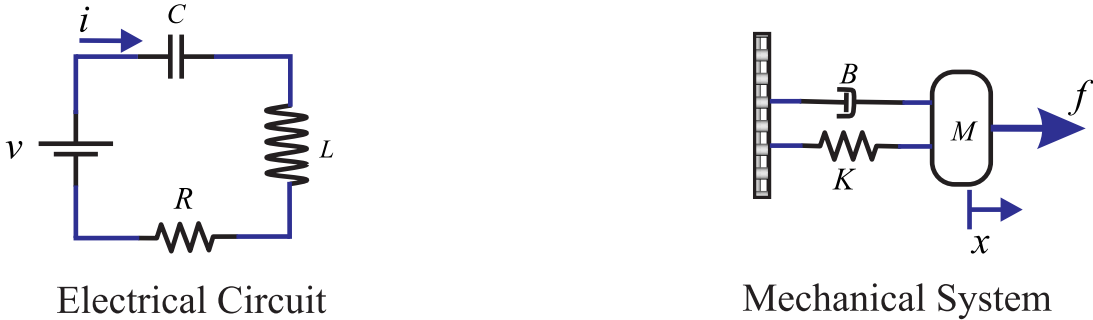
FIG. 9. A mechanical system and its equivalent electrical circuit. i represents the electrical current in the electrical system and x represents the displacement. By taking the velocity \dot{x} equivalent to the electrical current i , and appropriate values for each component in both the electrical circuit and the mechanical system, the output for both will be identical.
