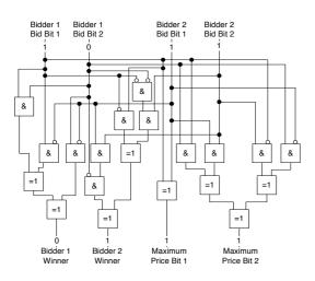
Figure 1: A Simple Auction Circuit. A & gate represents an AND gate and a = 1 gate represents an OR gate. Solid circles represent a join in the wires and unfilled circuits represent NOT gates.
