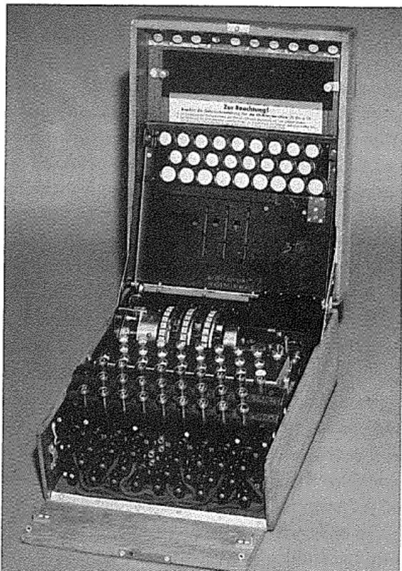
The process of cyphering is simple and quick. The message is 'typed' on a normal keyboard and as each letter is pressed, another letter is illuminated on a lampboard containing the 26 letters of the alphabet. The series of letters illuminated on the lampboard form the cypher text and the recipient of the cypher message, in possession of an identical machine, types out the cypher text and the decoded message appears on the keyboard.
