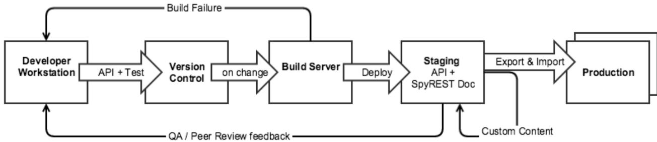
Fig. 2: API Development workflow using SpyREST at Cisco
