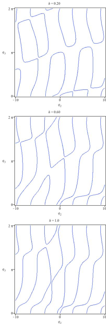
Fig. 4. Singularity locus bifurcation for HRR manipulator with respect to pitch parameter
