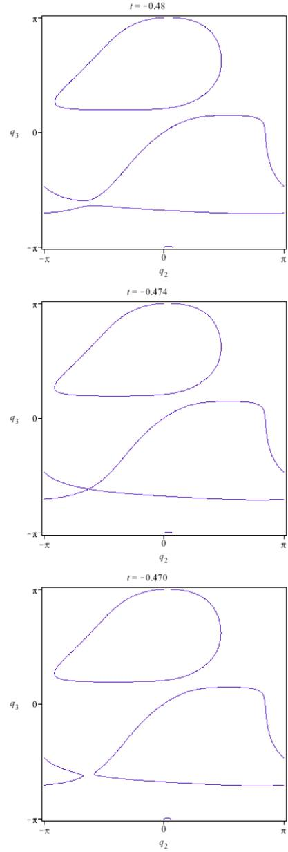
Fig. 3. Singularity locus bifurcation for a non-orthogonal 3R manipulator with respect to joint 3
