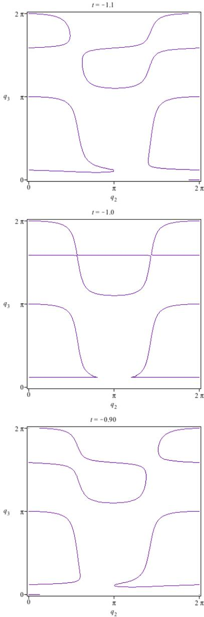
Fig. 2. Singularity locus bifurcation for an orthogonal 3R manipulator with respect to wrist centre
